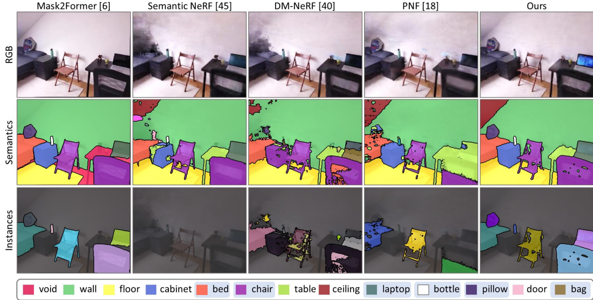
Figure 7. Novel views and their corresponding semantics and instances on in-the-wild room capture. Highlighted labels in the legend represent instanced ( thing ) classes. All 3D methods use the same posed RGB images and 2D machine-generated labels for training. PNF [19] additionally uses predictions from a 3D bounding box detector.
